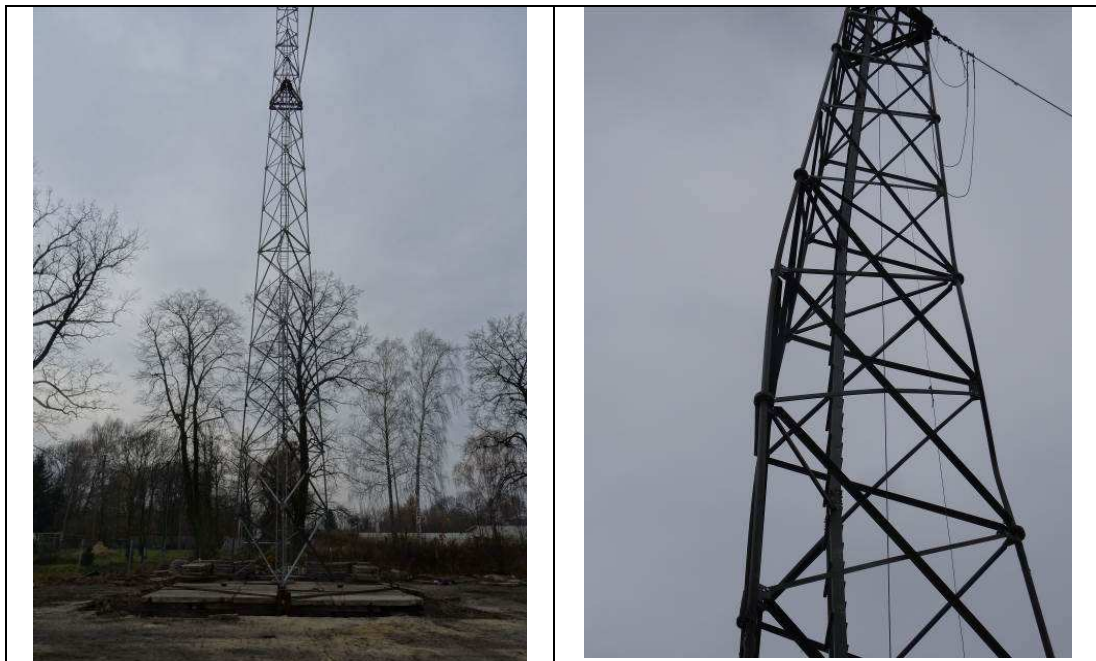
Figure 6: Failure mode of the first tested tower – view from the front (left) and the elevation (right)
