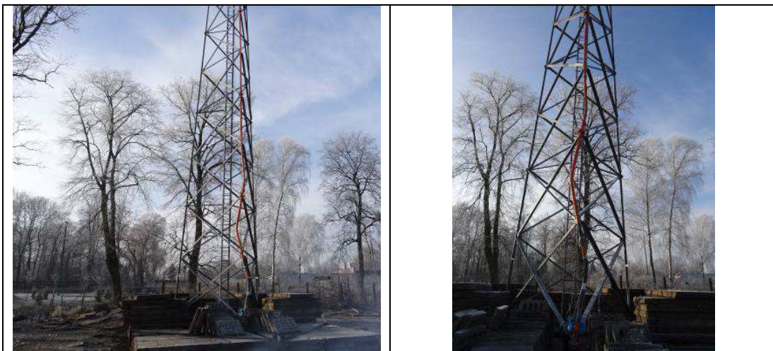
Figure 8: Buckling of tower legs in section S-7 (second test)
