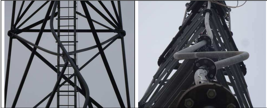
Figure 7: Buckling of tower legs in section S-5 (first test) – view from the front (left) and the base (right)
